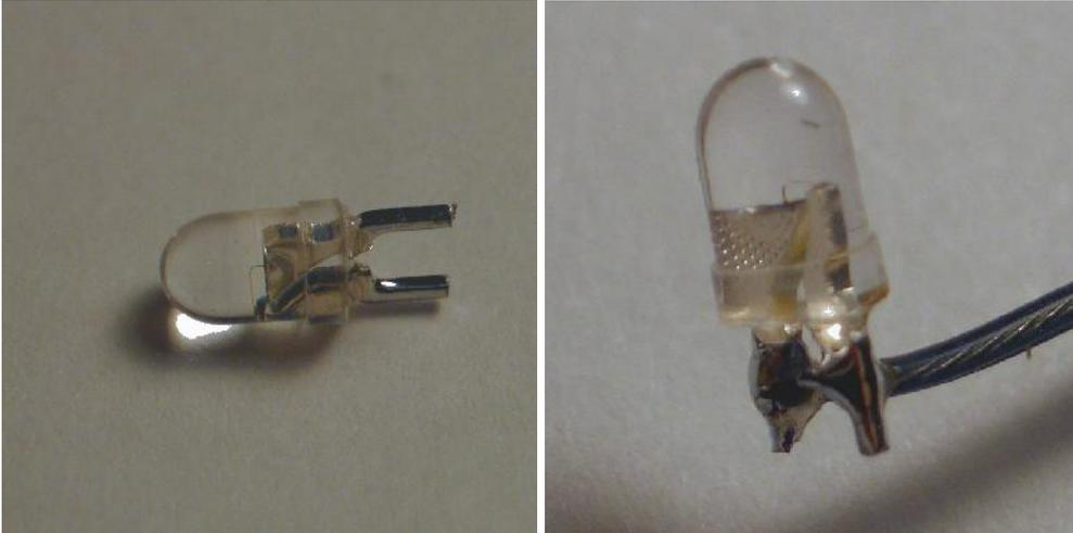
3. Insert the LEDs into their holders as shown below. The LED leads should be at or below the top surface of the LED holder. If solder or wires are preventing LED from seating fully into the LED holder trim them with clippers. Thread LED wires through the hole in the main module
