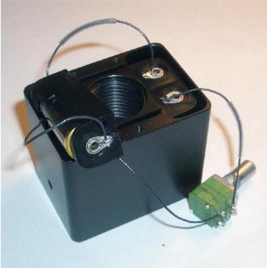
9. Insert the single battery holder into the main module body as shown. Push wires into channels on the main module body as shown. Insert the pot into the module cover as shown and **tighten the nut**. Tighten the cover to the main module body with three supplied screws. Turn the pot off (all the way counter clockwise) and place the pot knob as shown. Tighten the set screw on the knob. **Make sure that the knob is not touching the nut below and that the pot shaft rotates freely.**
