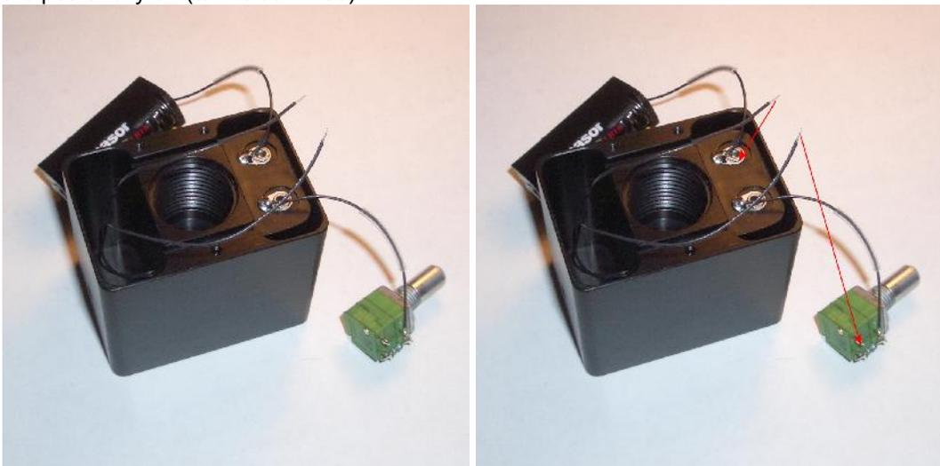
8. Solder the determined wire from LED to the terminal on the pot as shown. Solder the remaining wire to the bottom of the single battery holder as shown. **Please note the orientation of the wire soldered to the single battery holder. It must be exactly as shown because otherwise there will be a lot of strain on that wire.**
