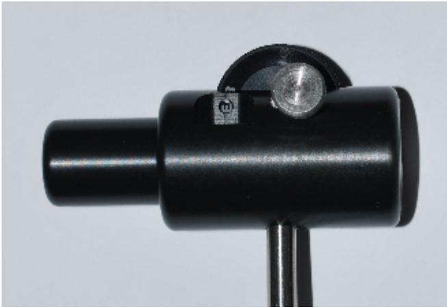
4. Take up slack on the probe cable so that it is routed through a cutout in the probe swivel fork. Carefully insert the probe and the main shaft into the cylinder. This is normally a close but loose fit. You should not have to use ANY force to insert the probe. If you encounter resistance please remove the probe and contact the factory.
