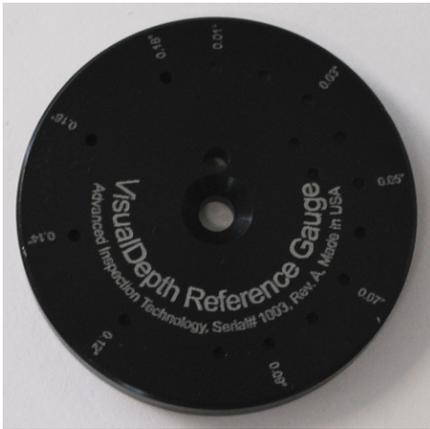
Please note that the reference gauge can be mounted to a fixed surface through a countersunk hole in the middle.
